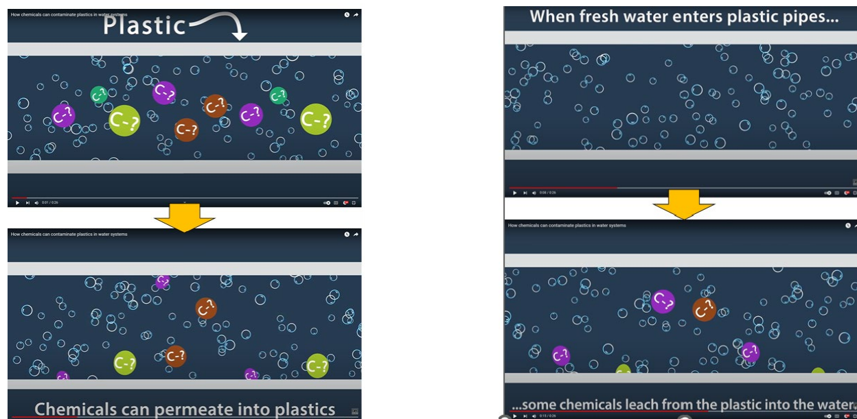
Figure 9. Stagnation before a water sample is collected helps chemicals leach from biofilms and infrastructure into the water, and this increases the chances contaminants present can be detectable by the laboratory method.
