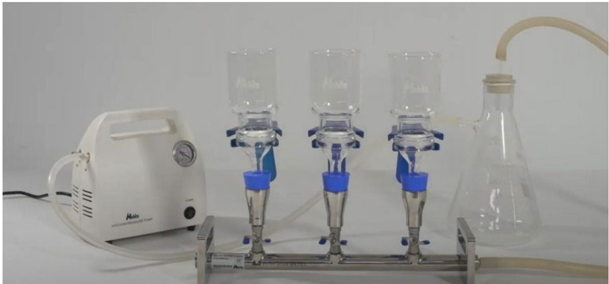
Figure B-2. Example Vacuum Manifold and Filtration Setup with Vacuum Pump.
