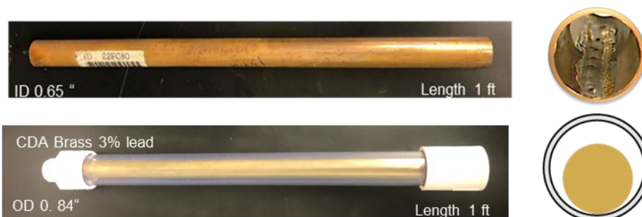
Figure 2-6. Pipe Materials Used for the Premise Plumbing Study.
