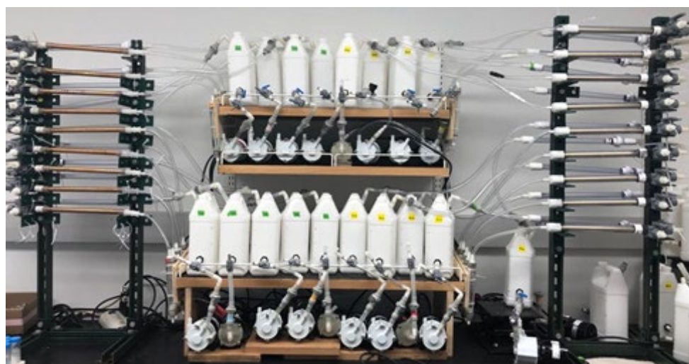
Figure 2-7. Laboratory Setup with Nine Loops of Copper Pipes Containing Lead Solder (left) and Nine Loops of Brass Rods within PVC Pipes (right).
