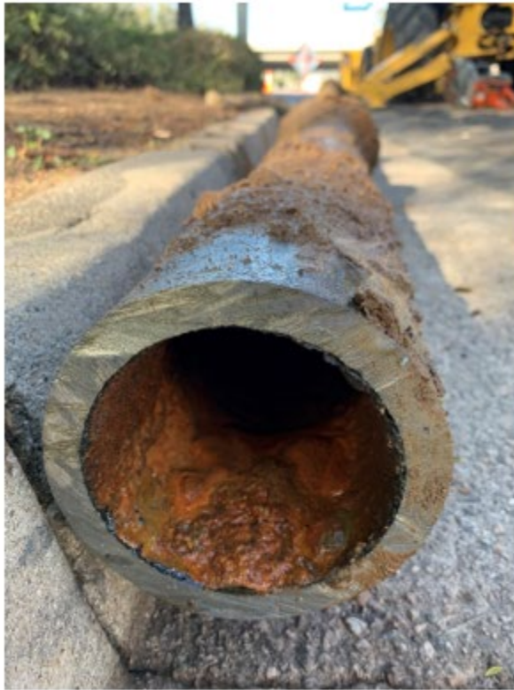
Figure 2-3. Unlined Iron Pipe Harvesting from the City of Pasadena with Visible Tuberculation and Deposits (left); Pipes Installed in the Pipe Loops at the MWD Demonstration Facility in Carson, CA (right).
