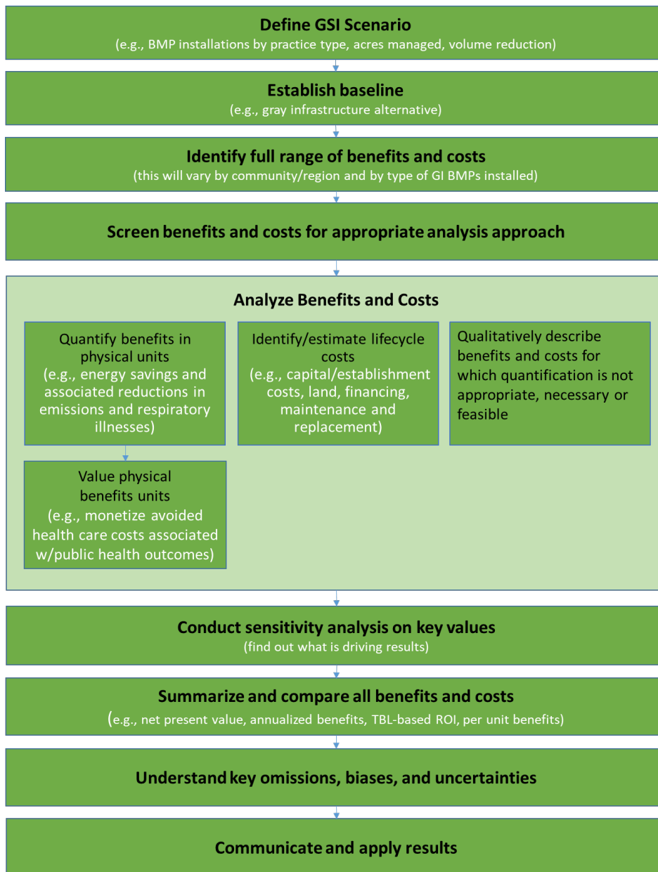
Figure ES-2. Economic Framework for Conducting TBL-Based Benefit Cost Analysis of GSI.
