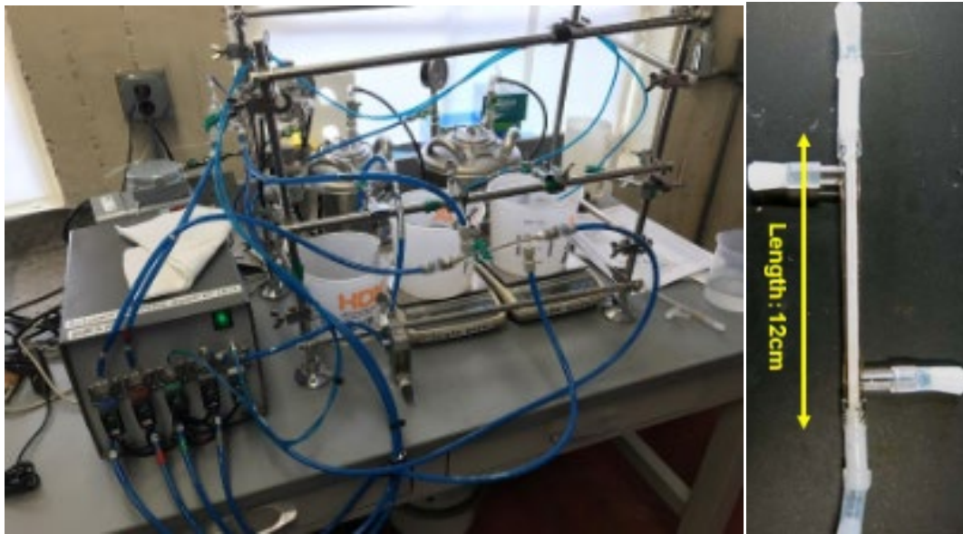
Figure 4-5. Bench-Scale MF/UF System Setup (left) and a UF Test Module (right).
