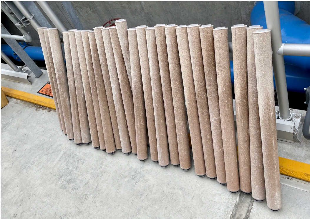
Figure 5-6. Cartridges After Changeout on January 28, 2021.
