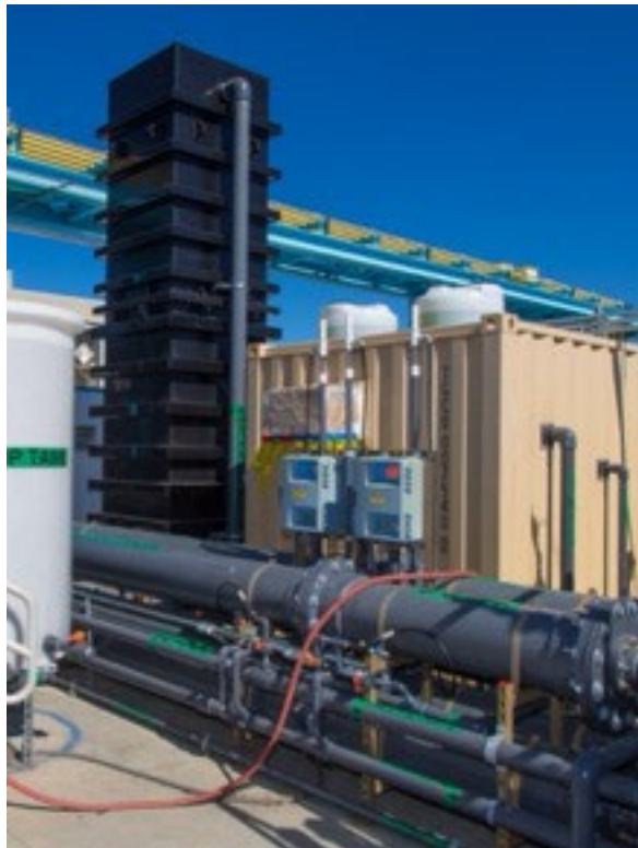
Figure 4-6. An Example Pilot-scale BAF System.
