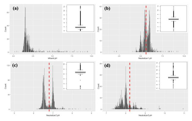
**Figure 2**. The pH performance of the existing neutralization process. The boxplots show the maximum, minimum, median, first quartile and third quantile values for influent and three neutralizer pH.
