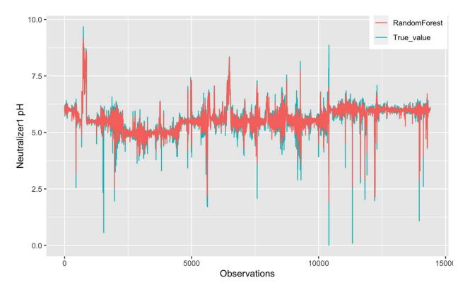
**Figure 4.** Predicted (red line) and actual (green line) pH of neutralizer #1 with the Random Forest regression model.
