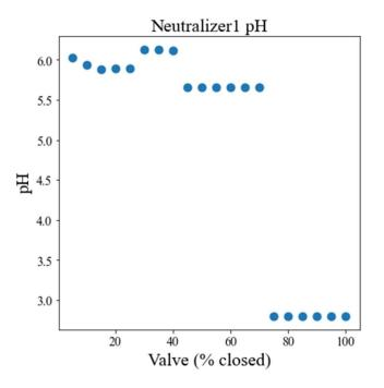
Figure 6. The recommended lime addition valve #1 position for neutralizer #1 pH
