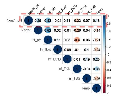
**Figure 3.** Correlation matrix among features for neutralizer #1. The color and size of circles, and values indicate the correlation between two features.
