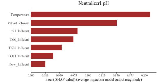
Figure 5. Sensitivity analysis of neutralizer #1 pH with the Random Forest regression model
