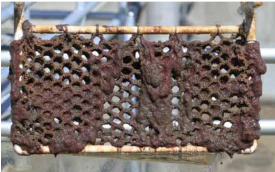
Figure 5 - Example of a Thick Biofilm on Fixed Rope Media
