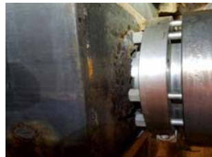
Carbon steel counterweight and stainless steel arm
