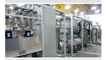
Hydrothermal processing (HTP) offers the ability to turn solids into renewable energy, using the same components that have long formed fossil fuels in nature (water, heat, and pressure), and speeding up the process so it takes place in about an hour, rather than several millions of years.
