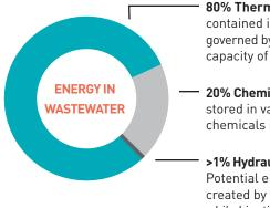
80% Thermal: Heat energy contained in wastewater, governed by the specific heat capacity of water.
