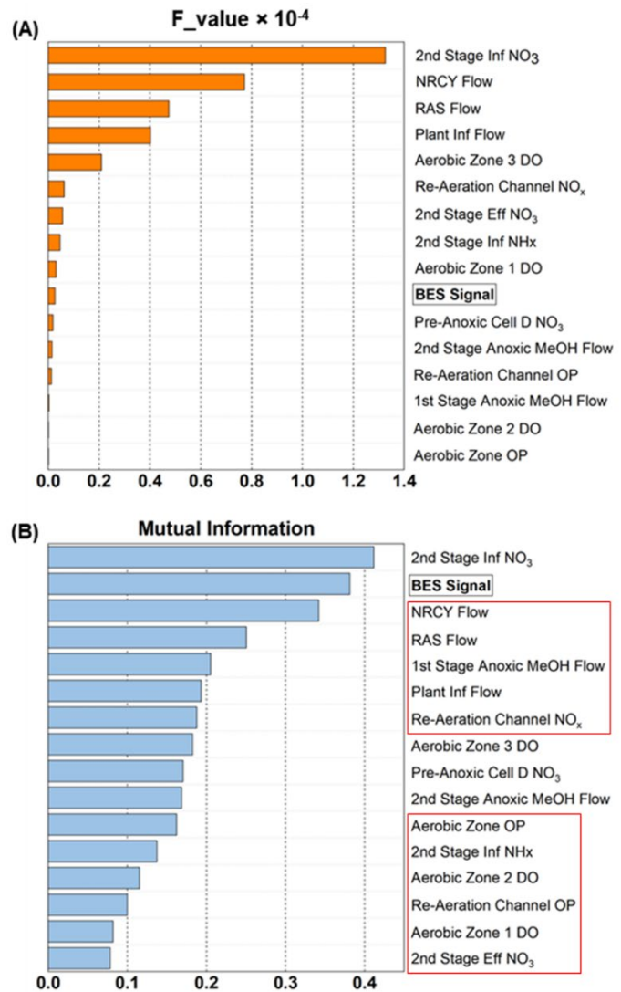
Figure 3. Linear correlation or F-test regression (A) and general information or MI analysis (B). The variables in the red box and the BES signal were selected as the final variables for development of the regression models.
